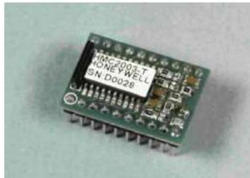
Figure 3: HMC2003 Magnetometer
